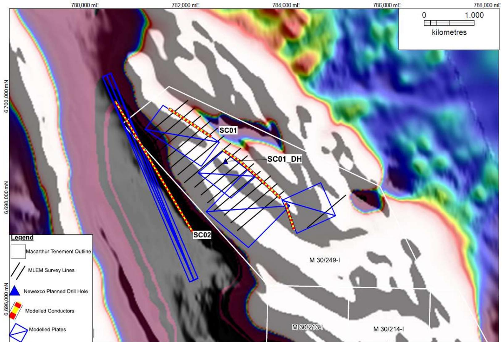
Figure 2. MLEM Survey at Snark showing modelled conductors. Background shows Total Magnetic Intensity anomalies
