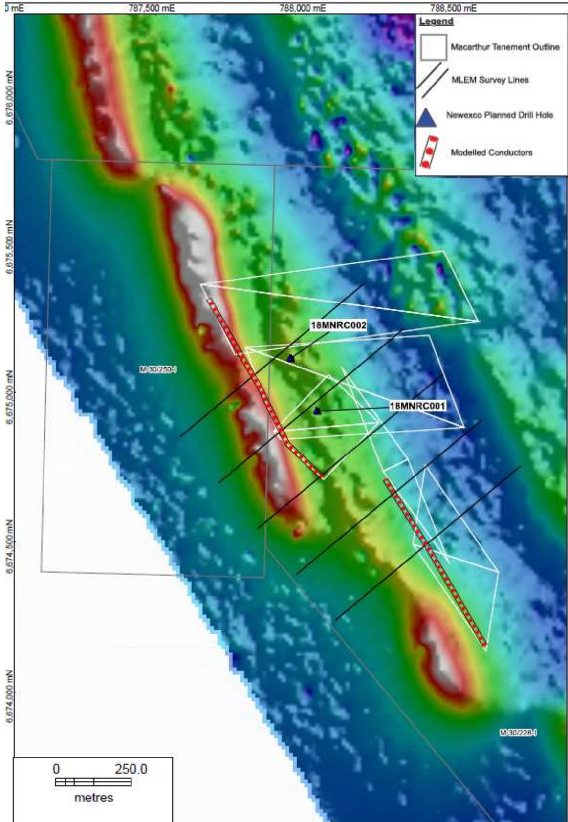
Figure 1. MLEM survey at Moonshine showing modelled conductors and location of RC drill holes. Background image shows magnetic anomalies.
